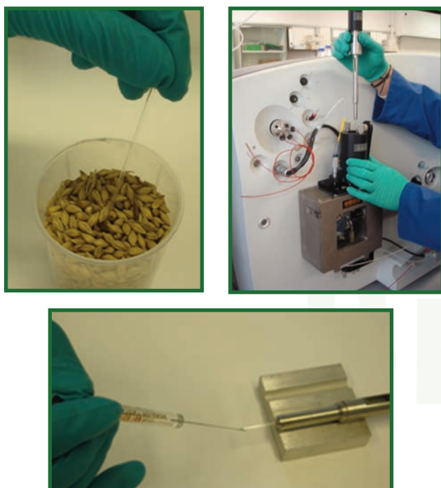
Figure 2. Analyses of a grain sample by ambient ionization mass spectrometry (ASAP) – Note the minimal sample preparation required.
